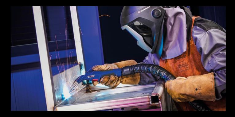
The xFUME® COMPACT fume extraction torch will quickly become a favourite tool when it comes to welding thin sheets and currents of up to 250 amperes are used. Weight, haptics and handling make it easy to forget that you have a welding fume extraction torch in your hand. The optionally short or long button additionally supports this feeling – while a leather covering tube not only protects the cable assembly, but also allows it to glide easily over edges.
