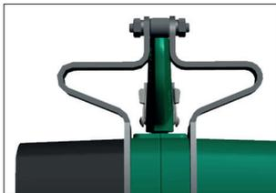
A redundant optional fall support capable of holding the maximum capacity of a hoist coming free of the supporting structure. The new limit switches offer another safety bonus. They will switch off the lifting and lowering movement as soon as the bumper touches the stop valve. This slows the movement and keeps the chain from being overloaded. All of these features enhance occupational safety significantly and minimize safety hazards and wear risks.
